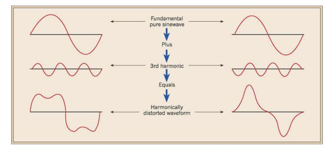
Harmonic distortion levels can be characterized by the complete harmonic spectrum with magnitudes and phase angles of each individual harmonic component. It is also common to use the Total Harmonic Distortion (THD), as a measure of the effective value
